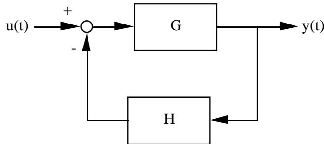
**Figure 2.5.** Block diagram showing the connection of two operators, where  $G$  is strictly passive (but otherwise arbitrary), and  $H$  is a system to which it is connected. Signals  $u(t)$  and  $y(t)$  do not have to be a complimentary effort/flow pair.
