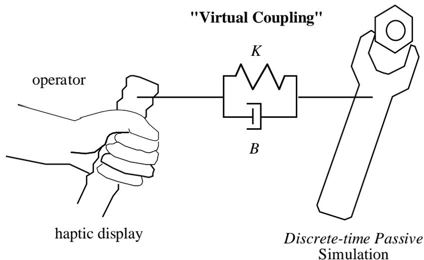
**Figure 3.4.** Conceptualization of a virtual coupling in a hand tool simulation.
