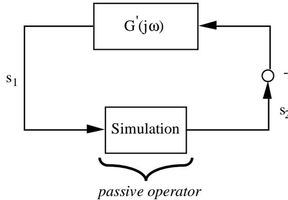
**Figure 4.2.** Coupled stability form of haptic display system. The mechanism, ALTIP impedance, sample/hold, and two-port virtual coupling dynamics are contained in  $G'(j\omega)$ . The virtual environment is restricted to be discrete time passive.
