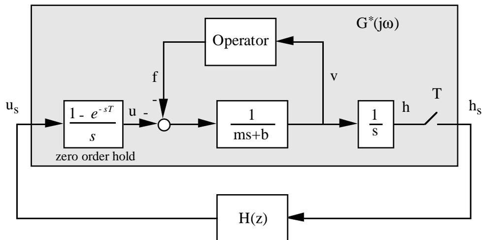
**Figure 3.1.** Colgate and Schenkel's model of a 1 DOF haptic display. Parameters  $m$  and  $b$  are the inherent inertia and damping of the haptic display handle.  $H(z)$  is the virtual environment,  $T$  is the sample time,  $h$  is the handle position and  $u$  is the actuator effort ( $h_s$  and  $u_s$  after sampling).
