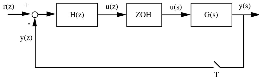
**Figure 2.2.** Block diagram of a linear sampled-data system with a zero order hold and periodic sampling. Continuous functions are represented in the Laplace domain with  $f(s)$ , and discrete functions are represented with  $f(z)$ .
