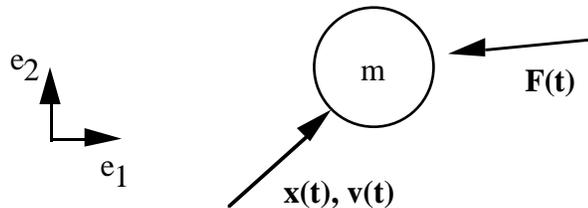
**Figure 5.4.** Two DOF particle, with position  $\mathbf{x}(t)$  and velocity  $\mathbf{v}(t)$ , and an arbitrary force  $\mathbf{F}(t)$  acting on it (note that  $\mathbf{x}(t)$ ,  $\mathbf{v}(t)$  and  $\mathbf{F}(t)$  are all vectors).
