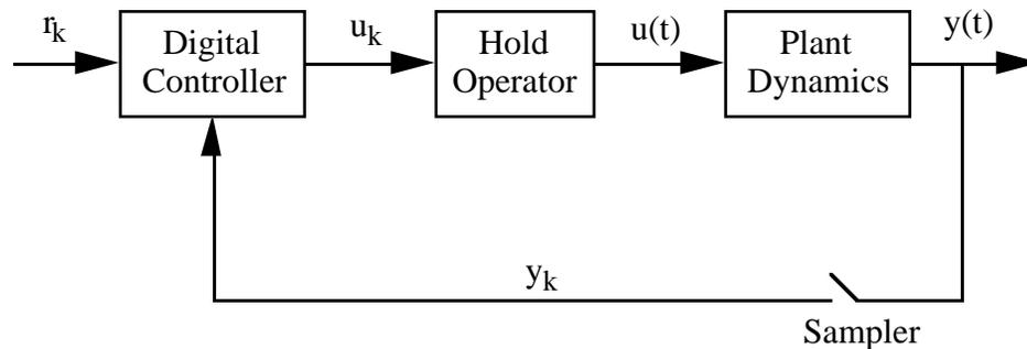
**Figure 2.1.** Diagram of a sampled data system. Continuous functions are represented with  $f(t)$ , whereas discrete functions are represented with  $f_k$ . The computed controller effort,  $u_k$ , becomes a continuous signal,  $u(t)$ , through the hold operator. The plant output,  $y(t)$ , is sampled, becoming  $y_k$ . In addition to the plant output, the digital controller acts on the discrete reference signal  $r_k$ .
