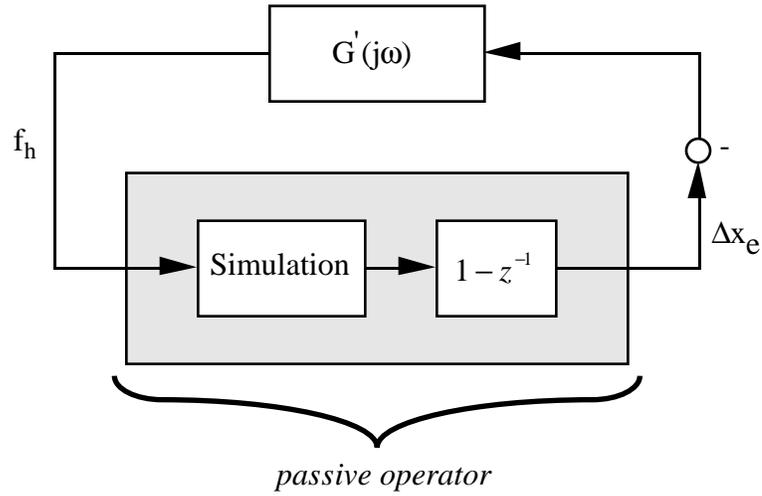
**Figure 4.4.** Coupled stability form of haptic display system. The mechanism, ALTIP impedance, sample/hold, and one-port virtual coupling dynamics are contained in  $G'(j\omega)$ . The virtual environment is restricted to be discrete time passive.
