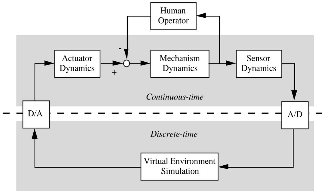
**Figure 2.4.** Generic block diagram a haptic display. The human, actuators, mechanism, and sensors are all continuous-time systems, while the virtual environment is a discrete-time system. The A/D and D/A form the interface between them. The shaded areas emphasize which parts of the haptic display are continuous vs. discrete time.
