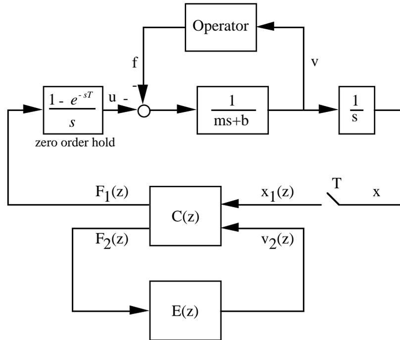
**Figure 3.5.** Block diagram of a 1 DOF haptic display using a virtual coupling. The virtual coupling and environment are represented by  $C(z)$  and  $E(z)$ , respectively. The human operator, as in previous work, is replaced with an arbitrary linear time-invariant passive operator.
