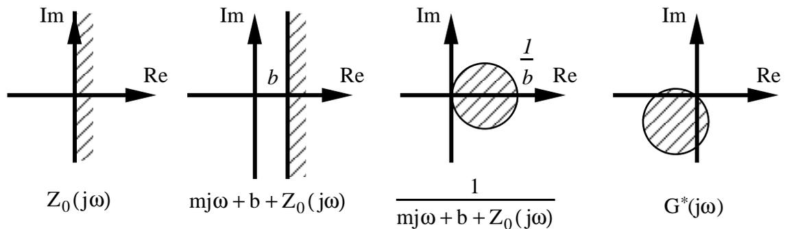
**Figure 3.2.** Graphical representation of passivity derivation. Regions corresponding to the ALTIP impedance, mechanism, and sample/hold dynamics are shown in the Nyquist plane.
