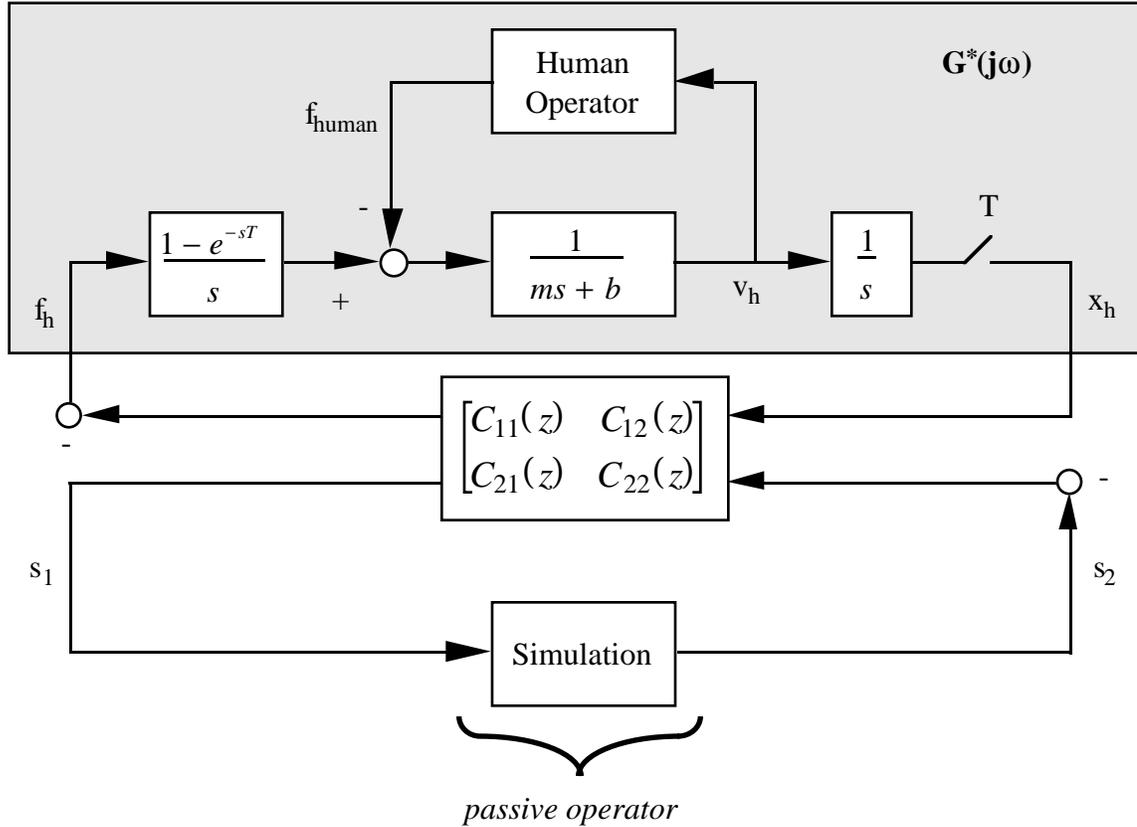
**Figure 4.1.** Model of a haptic display with a two-port virtual coupling.  $G^*(j\omega)$  represents the dynamics of the sample/hold, mechanism, and human operator,  $x_h$  is the measured position of the haptic display handle, while  $f_h$  is the force to be applied to the mechanism by the actuators. Signals  $s_1$  and  $s_2$  are the inputs and outputs of the simulation, and are not required to be specified for the analysis.
