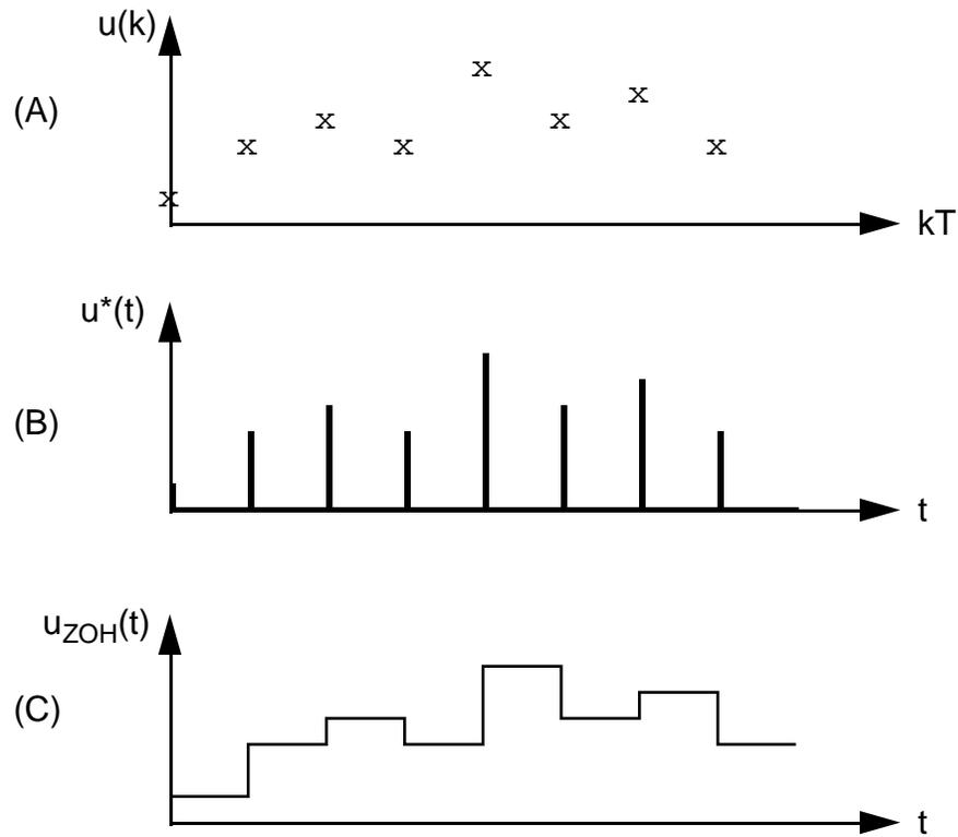
**Figure 2.3.** Representations of discrete signals. Original discrete signal (A), pulse variable description (B), signal after zero order hold (C).
