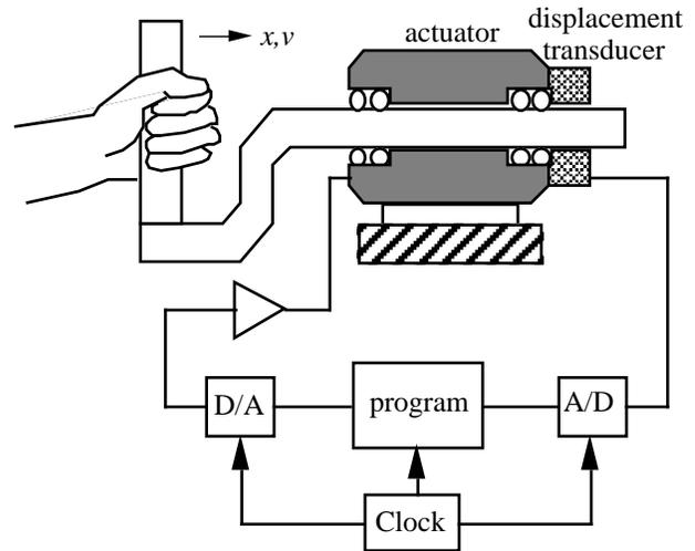
Figure 1. Schematic of a one degree-of-freedom haptic interface.
