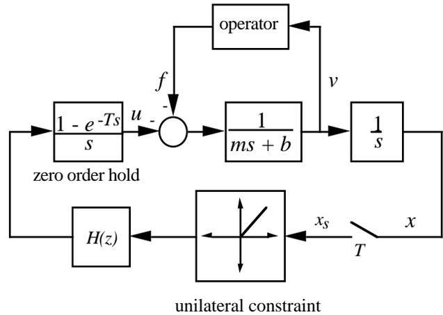
Figure 2. Model of a one degree-of-freedom haptic interface.  $m$  is the inherent mass of the display,  $b$  is inherent damping,  $v$  is velocity,  $x$  is position,  $x_s$  is the sampled position,  $T$  is the sampling rate,  $u$  is the control effort, and  $f$  is the force applied by the operator.
