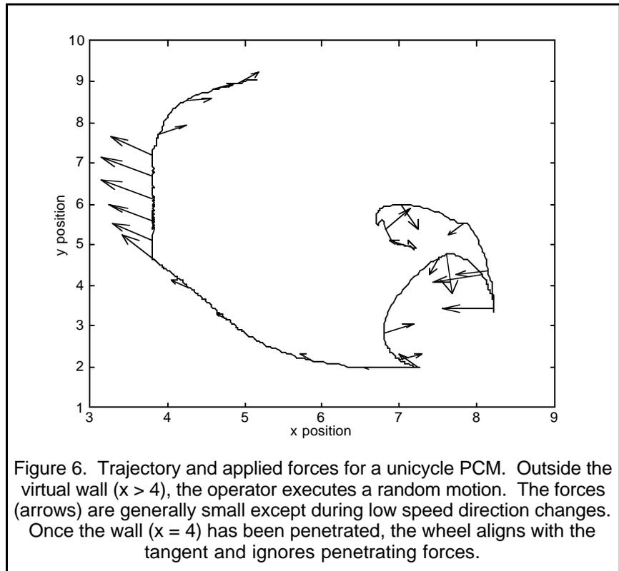
Figure 6. Trajectory and applied forces for a unicycle PCM. Outside the virtual wall ( $x > 4$ ), the operator executes a random motion. The forces (arrows) are generally small except during low speed direction changes. Once the wall ( $x = 4$ ) has been penetrated, the wheel aligns with the tangent and ignores penetrating forces.
