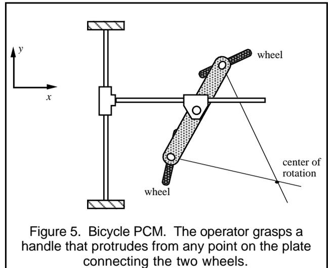
Figure 5. Bicycle PCM. The operator grasps a handle that protrudes from any point on the plate connecting the two wheels.
