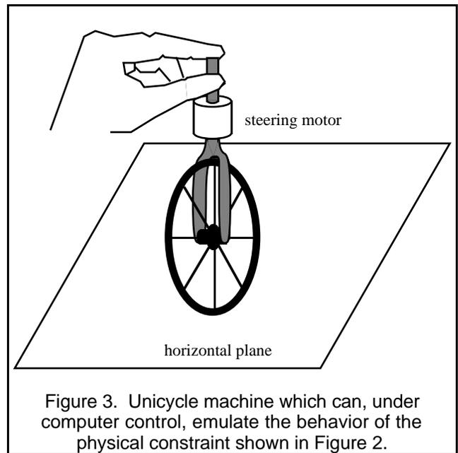
Figure 3. Unicycle machine which can, under computer control, emulate the behavior of the physical constraint shown in Figure 2.
