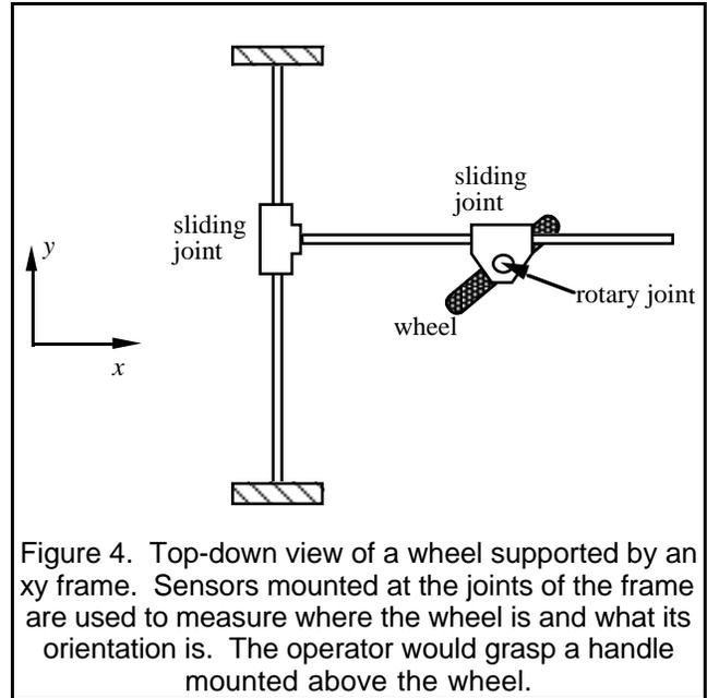
Figure 4. Top-down view of a wheel supported by an  $xy$  frame. Sensors mounted at the joints of the frame are used to measure where the wheel is and what its orientation is. The operator would grasp a handle mounted above the wheel.
