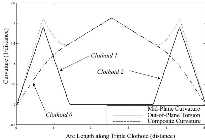
**Figure 10.** Mid-plane curvature, out-of-plane torsion and composite curvature are plotted versus path length of the triple-clothoid.
