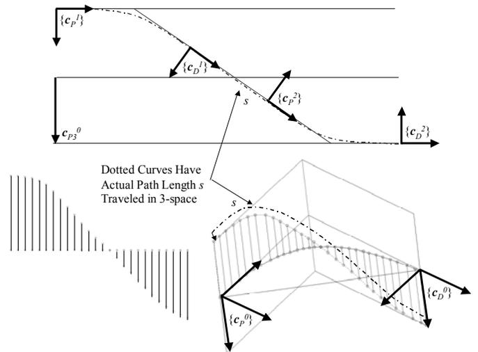
**Figure 6. Local coordinate frames for the proximal and distal portions of each clothoid are represented by  $\{c_p^0\}$ ,  $\{c_D^0\}$ ,  $\{c_p^1\}$ ,  $\{c_D^1\}$ ,  $\{c_p^2\}$  and  $\{c_D^2\}$  frames as defined in the Appendix. The  $c_{p3}^0$  unit vector is**
