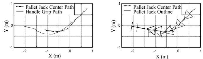
**Figure 13. Pallet Jack Path and Handle Path. The solid line of the left plot shows the trace of the handle grip. In the right plot of Fig. 13, an outline of the Pallet Jack Cobot and its handle is shown at half-second intervals.**
