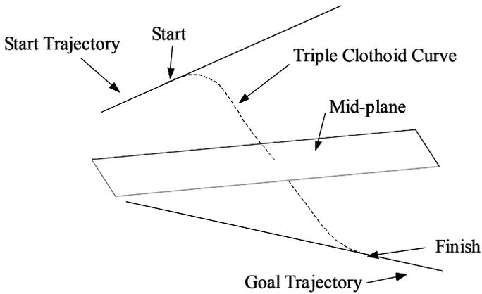
**Figure 3. A triple-clothoid trajectory branches off of the start trajectory and merges with the goal trajectory at the start and finish points respectively. A mid-plane is defined by a normal that is the shortest distance between the two non-intersecting trajectories.**
