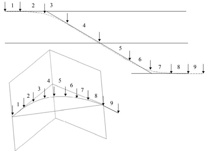
**Figure 11.** The nine possible segments of a triple-clothoid curve. Note that either segments *1* and *8* will have zero length (case represented in Fig. 8) or segments *4* and *5* will have zero length (case represented in Fig. 9). Figure 11 as drawn does not represent either case since all nine segments have finite length for the purpose of illustration.
