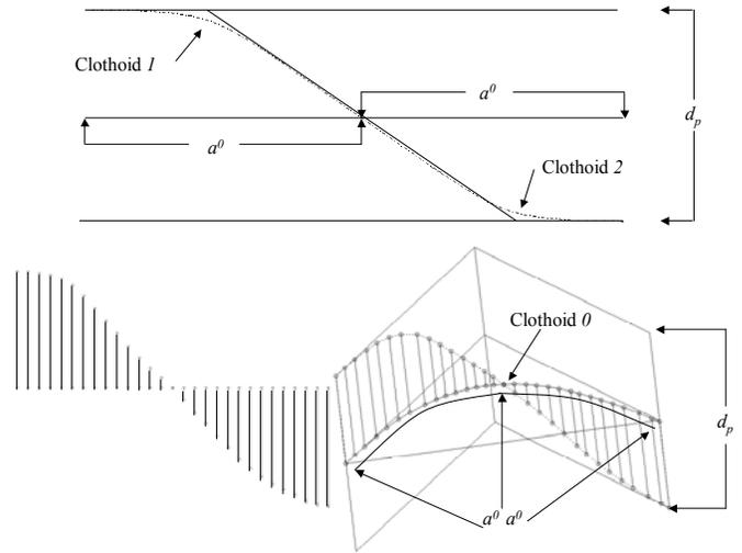
**Figure 5. The surface defined by the lines of projection (lower right) is laid flat (lower left) in a plane without distortion of surface area. Arc-length  $a^0$  and shortest perpendicular distance  $d_p$  are preserved (upper). *Clothoid 0* is delineated in the mid-plane (lower right) and *Clothoids 1* and *2* in the flattened surface (upper).**
