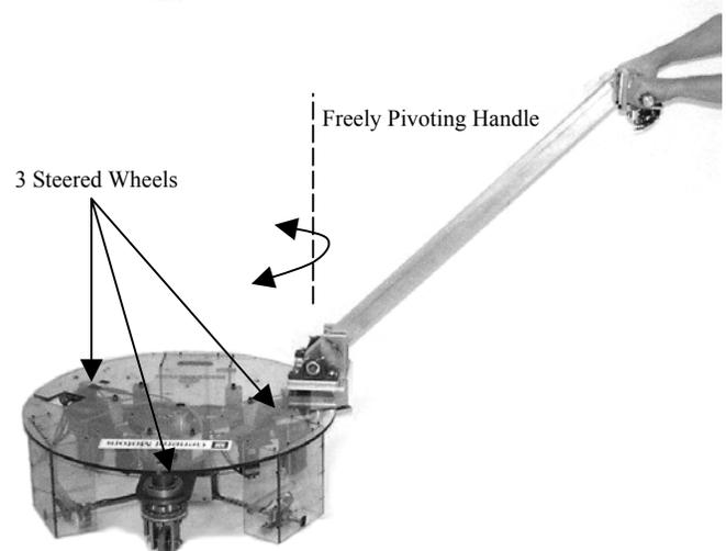
**Figure 1.** A handle that is fixed vertically and pivots freely in the horizontal plane is added to the three-wheeled “Scooter Cobot” to create a “Pallet Jack Cobot.” The wheels are steered by computer control in response to the handle angle or presence of a constraint surface but remain un-powered about their rolling axes.
