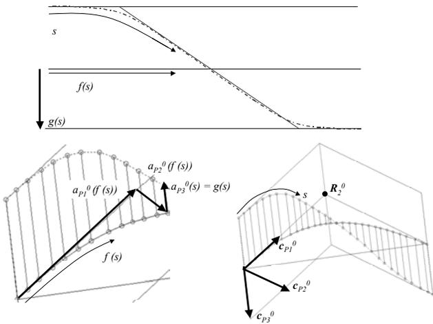
Figure 7. The local frames of *Clothoids 1* and *2* map actual path-length  $s$  to  $f(s)$  and  $g(s)$  which are orthogonal to *Clothoid 0* local frames. *Clothoid 0* local frame coordinates can then be transferred to the global frame. Thus *Clothoid 0* proximal frame coordinates are the following functions of  $s$ ;  $a_{P1}^0(f(s))$ ,  $a_{P2}^0(f(s))$  and  $a_{P3}^0(s)=g(s)$ .
