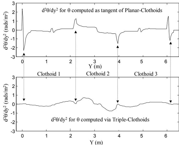
**Figure 15. A user of the Pallet Jack Cobot experiences lower linear accelerations and jerks when the triple-clothoid solution to three-dimensional trajectory generation is used in preference to a modified planar-clothoid solution.**
