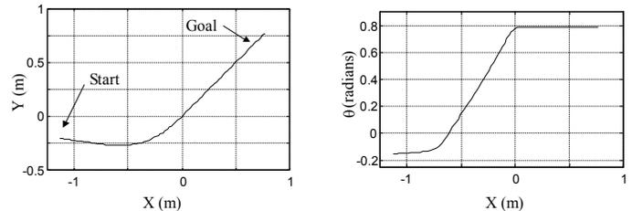
**Figure 12. Two projections of a three-dimensional triple-clothoid trajectory for the  $x-y-\theta$  Pallet Jack Cobot.**
