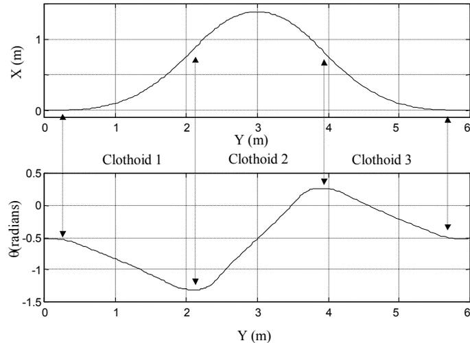
**Figure 14. Three triple-clothoids chained together to form a dodge maneuver.**
