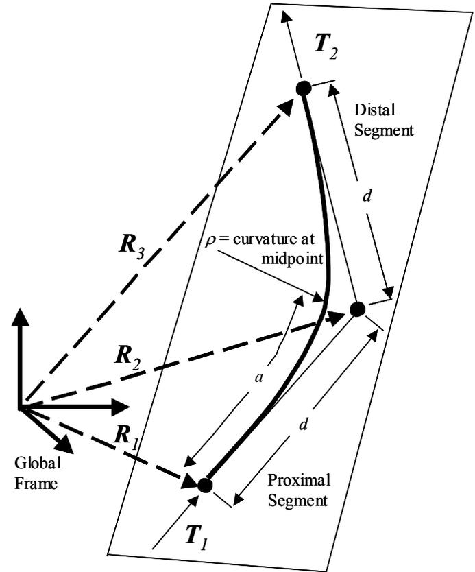
Figure 2. The planar-clothoid geometry consists of two control points  $R_1$  and  $R_3$ , at which start and goal tangents  $T_1$  and  $T_2$  are defined.
