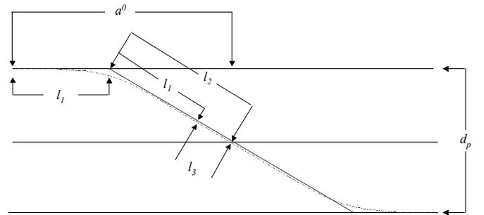
Figure 8. The first case for  $l_1/a^0$  is chosen such that  $l_1 < l_2$ ,  $l_3 = l_2 - l_1$ , and  $l_4 = 0$ .
