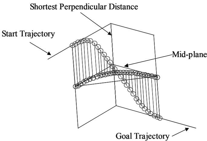
**Figure 4. Two planes that are normal to the mid-plane and parallel to the start trajectory and goal trajectory respectively, are added to the construction. Lines of projection from the triple-clothoid curve to the mid-plane are also shown.**
