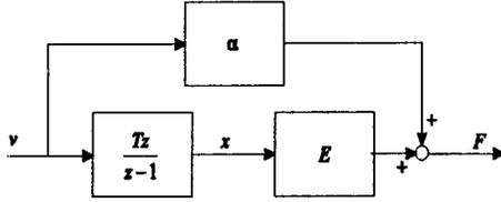
Figure 7: Environment block with parameter  $\alpha$ . The mapping from velocity to force must be passive.
