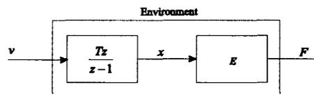
Figure 3: Discrete-time block diagram representing nonlinear stiffness. The environment block consists of an integrator and static nonlinear operator  $E$ .
