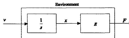
Figure 2: Continuous-time block diagram representing nonlinear stiffness. The environment block consists of an integrator and static nonlinear operator  $E$ .
