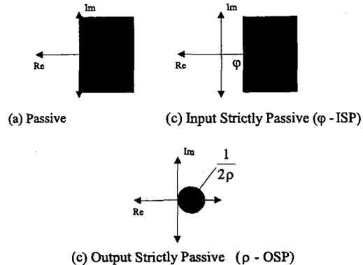
Fig. 2. Frequency domain interpretations of the different levels of passivity.
