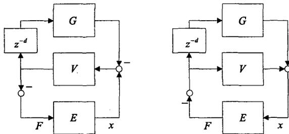
Fig. 1. Admittance and Impedance implementation block diagrams.
