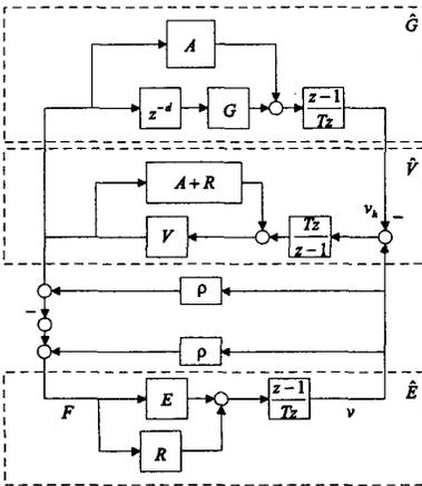
Fig. 5. Transformed haptic system with admittance environment.
