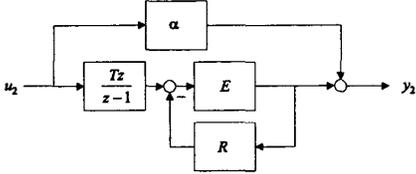
Fig. 7. Impedance environment block. The mapping from  $u_2$  to  $y_2$  must be passive.
