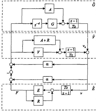
Fig. 4. Transformed haptic system with impedance environment.
