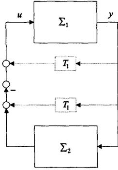
Fig. 3. Loop transformation of Coupled System.
