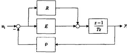
Fig. 6. Admittance environment block. The mapping from  $u_1$  to  $y_1$  must be passive.
