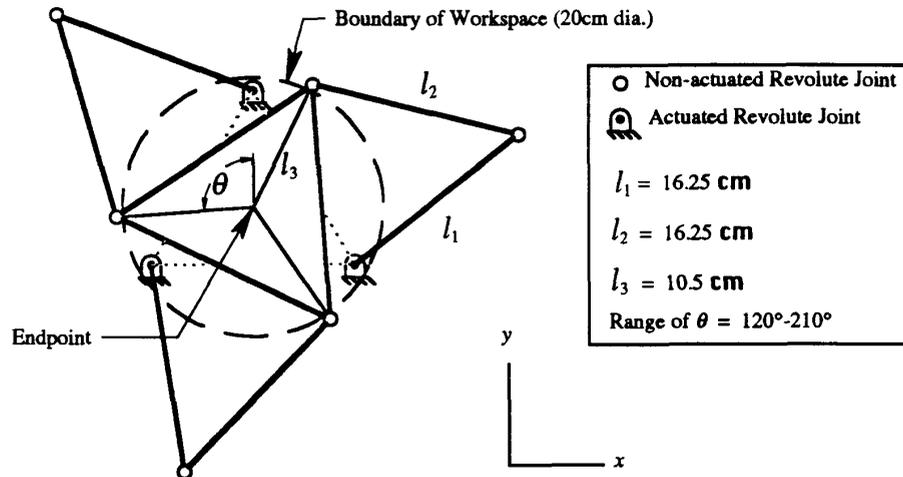
Figure 2. Kinematic diagram of planar, parallel-link mechanism.
