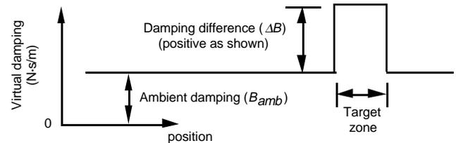
FIGURE 2. Virtual damping vs. handle position. The independent variables in all of the experiments were ambient damping ( $B_{amb}$ ) and damping difference ( $\Delta B$ ). In a block of trials, targets appeared once at each of nine discrete locations throughout the workspace. The order of appearance of these nine locations was random.
