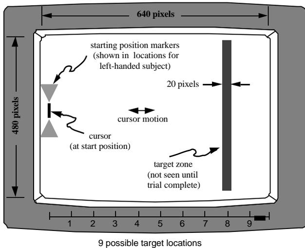
FIGURE 3. CRT display for Experiments 1, 2, and 3. Starting position markers and target zone shown in proper arrangement for left-handed subject.
