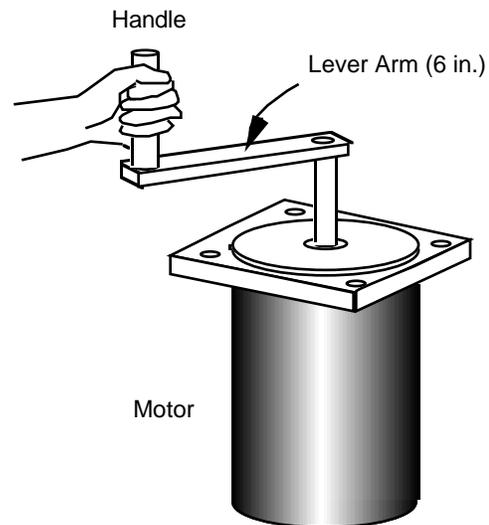
Figure 1(a). Sketch of one degree-of freedom "crank" manipulandum used in experiments.
