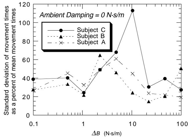
FIGURE 5. Standard deviations of movement times (normalized by mean movement times) vs. damping difference. Cases shown are for ambient damping equals zero.
