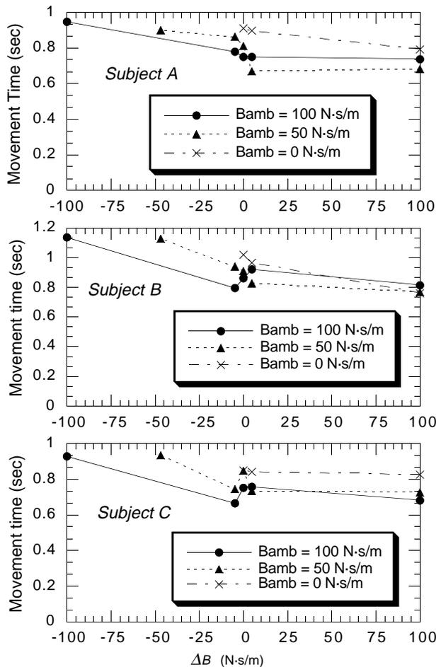
FIGURE 6. Average movement times for Experiment 2, positioning with visual feedback of target position, for all three subjects.
