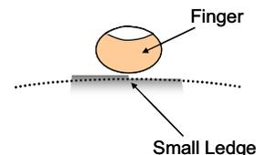
Figure 2: A small ledge runs the periphery of the rotating contact wheel, serving as the feature. The motion of the wheel as pictured is in (or out) of the page.
