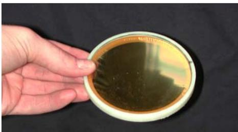
Figure 1: The Mechanical filter is made of a thin sheet of Kapton bound between two concentric rings of nylon.
