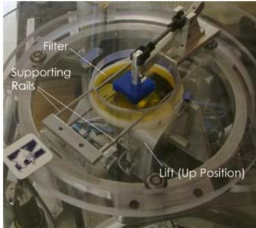
Figure 3: Supporting rails hold the filter in place between the subject's finger and the rotating contact wheel.
