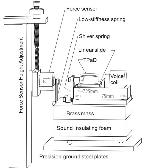
Fig. 3. The ShiverPaD device and the force sensing system.
