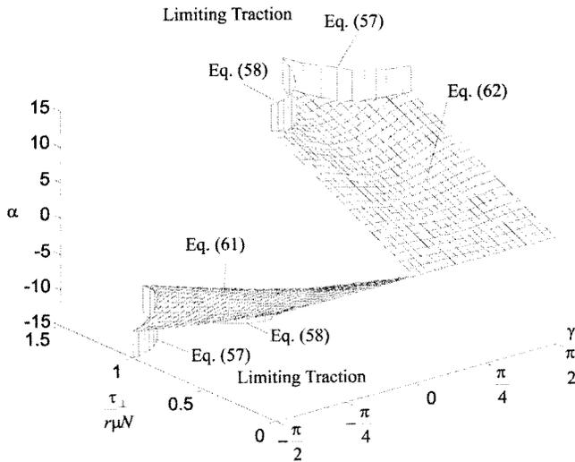
**Fig. 11 Sideslip angle  $\alpha$  as a function of the disallowed force  $\tau_{\perp}$  and the transmission angle  $\gamma$ . Beyond the limiting curve,  $\alpha$  will increase without regard to  $\tau_{\perp}$  applied.**
