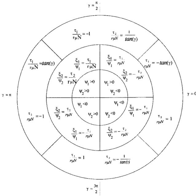
Fig. 9 The governing relationships are drawn graphically around a circle so as to indicate the range of  $\gamma$  in which they are valid. In concentric regions starting at the center, the signs of the spin parameters, the relationships between the creep to spin ratios and the drive roller torques, and the drive roller torque values at limiting friction are noted.
