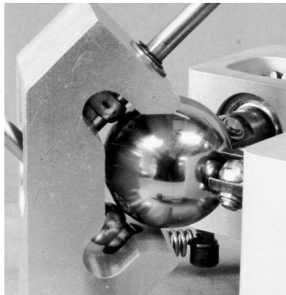
**Fig. 1** Photograph of the prototype CVT. The drive rollers with axes in the vertical plane are visible on the left while the steering rollers with axes in the horizontal plane are visible on the right.
