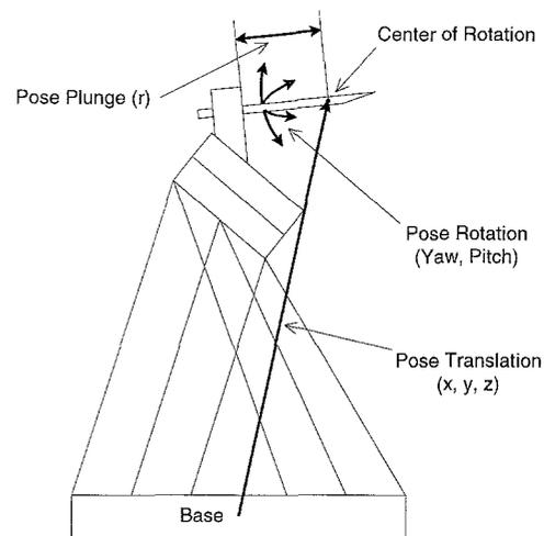
**Fig. 2** The pose definition of the manipulator includes six variables to define five degrees of freedom. The pose variables can be grouped into two sets of three variables each. One set locates the center of rotation with respect to the base in cartesian  $(x, y, z)$  coordinates. The other set describes the amount of rotation (yaw, pitch) and the plunge distance ( $r$ ) of the hypodermic needle with respect to the center of rotation
