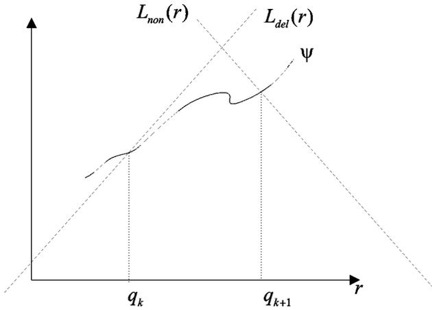
Fig. 6. Function  $L(r)$  bounding the nonlinearity over the interval  $(q_k \rightarrow q_{k+1})$ . The slope changes depending on whether the implementation is delayed or nondelayed.
