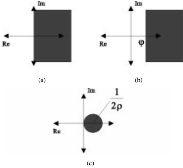
Fig. 2. Frequency-domain interpretations for the different levels of passivity: (a) passive; (b) input strictly passive ( $\psi$ -ISP); and (c)  $\rho$ -output strictly passive ( $\rho$ -OSP).
