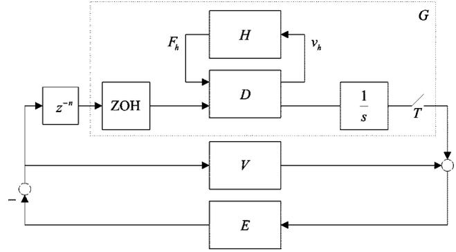
Fig. 3. Haptic system consisting of human ( $H$ ), haptic device ( $D$ ), virtual coupling ( $V$ ), and virtual environment ( $E$ ).
