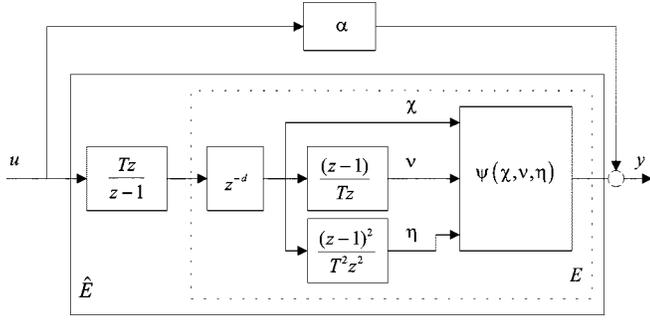
Fig. 5. Transformed environment block. Setting  $d = 0$  represents nondelayed implementation while setting  $d = 1$  represents delayed implementation.
