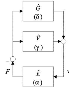
Fig. 4. Transformed haptic system.  $\hat{G}$  is the transformed version of human/device,  $\hat{V}$  is the transformed version of the virtual coupling, and  $\hat{E}$  represents the transformed environment.
