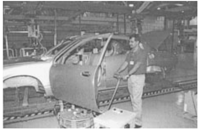
Fig. 6. GM's cobot is a rugged yet highly maneuverable device. It assists in removing doors from newly painted auto bodies prior to assembly of the cabin. This task was chosen because it was both difficult and slow for workers to remove the doors manually without marring the surfaces: the curvature and styling of the body panels is such that a specific "escape trajectory" is needed to remove the door safely. Human versatility and dexterity are still very important in other phases of the task; this is not a task that should be fully automated. The door-unloader cobot glides easily on servo-steered Rollerblade wheels with only a few pounds of operator force. During some task phases the operator controls position while the cobot controls orientation, aligning itself to the car body or to the door rack across the walkway as appropriate. In close-approach phase a virtual surface is created close to the vehicle's rocker panel, guiding the cobot to the correct location to grip the door without colliding with the vehicle. The "escape trajectory" is executed in path mode. When crossing the walkway the cobot is in free mode, giving the operator direct and intuitive control over both translation and orientation.
